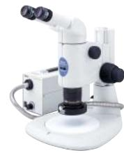
SMZ1500 configured with C-FIR Fiber-optics Ring Illuminator
