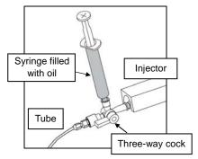
As shown, fix the three-way cock between the injector and tube, and also fix the syringe to the three-way cock.
