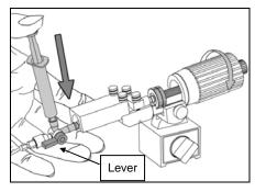
Turn the lever of the three-way cock in the direction as shown, fill oil in the syringe on the injector.
