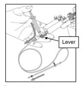
Turn the lever of the three-way cock in the direction as shown, fill oil in the tube/injection holder.
