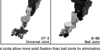
Universal joints allow more solid fixation than ball joints by eliminating other movement than tilt and pivot. The tilt and pivot movements are offered with the stopper mechanism which confines movement range. The stopper mechanism can reduce the possibility of accidental breakage of the pipette and also allows for return to the original position. (Stopper Function)
