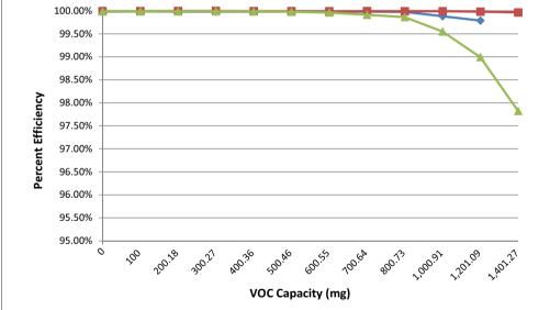
Results from testing 3 different UltraPure filters
