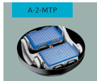
Swing-bucket rotor for 2 plates (MTP, PCR and deepwell plates) (max. 2,204 × g / 4,680 rpm)
