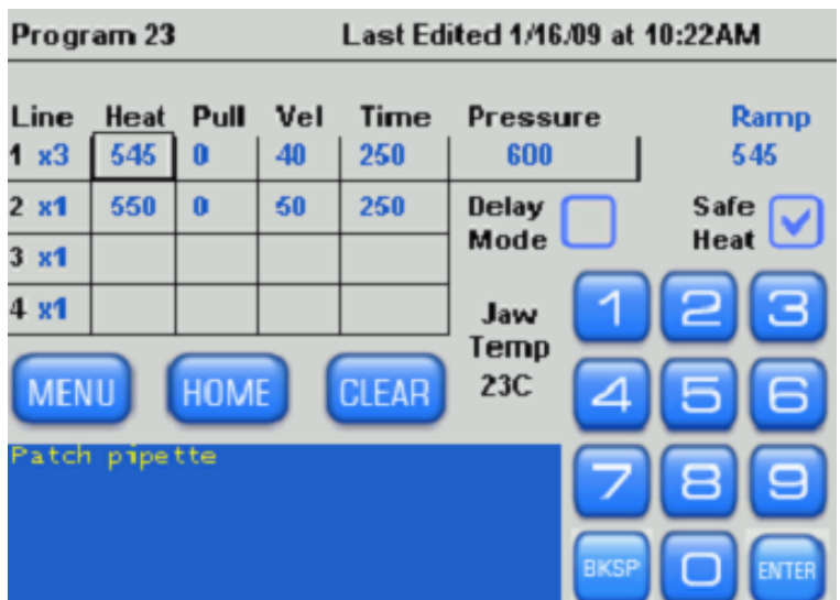
Figure 13. Two-line program with first line looped.
